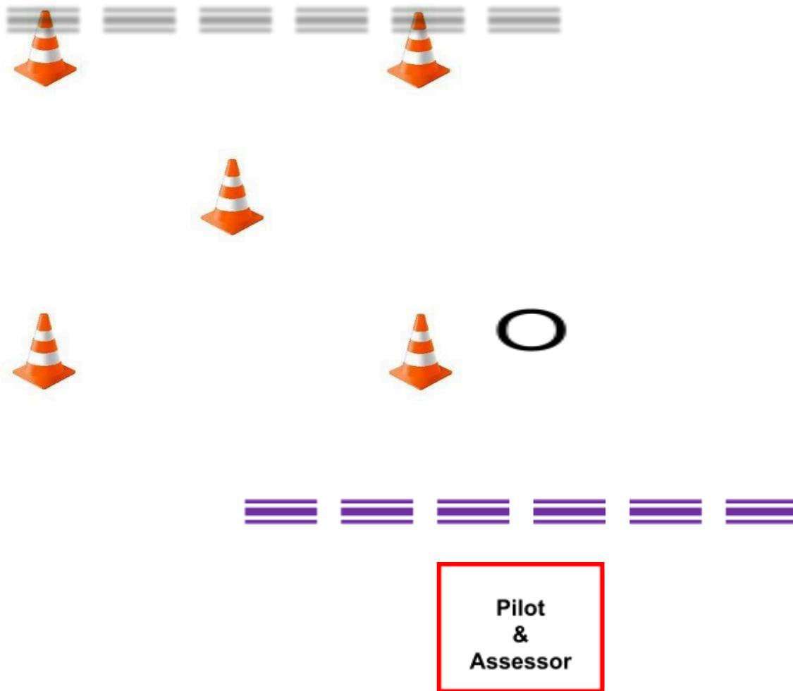
During the flight test, the assessor will direct the pilot to fly the aircraft to specific cones in differing sequences while conducting a range of manoeuvres. Instruction will also include different orientations and elevations of the aircraft as required.
